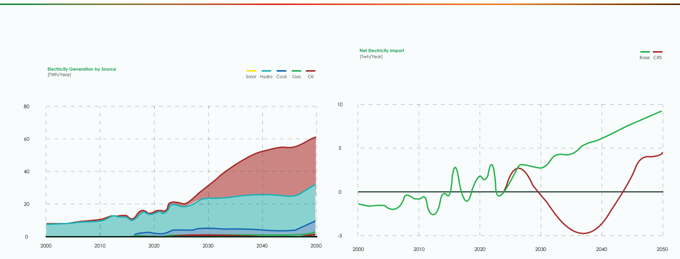
Figure 3.14: Electricity generation by source in the CRS scenario (left) and net electricity imports in Twh/yr, a positive representing import and negative corresponding to exports
